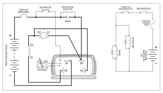
Fig. 10 Basic wiring configuration, Curtis PMC 1231C controller.
