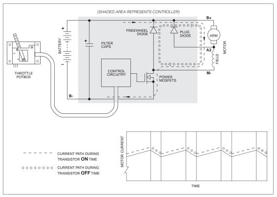
Fig. B-1 Pulse width modulation.
