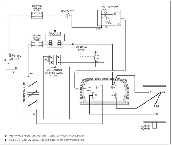
Fig. 8 Typical installation, Curtis PMC 1231C controller.
