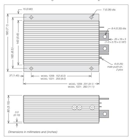
Be sure to mount the 1209B/1221B/1221C controller so as to allow access to the adjustment screws. Although not usually necessary, a thermal joint compound can be used to improve heat conduction from the case to the mounting surface.
