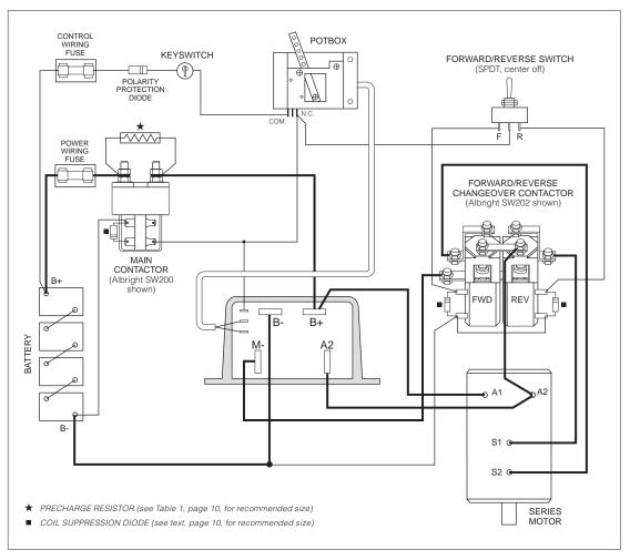
Fig. 7 Typical installation, Curtis PMC 1209B/1221B/1221C controllers.
