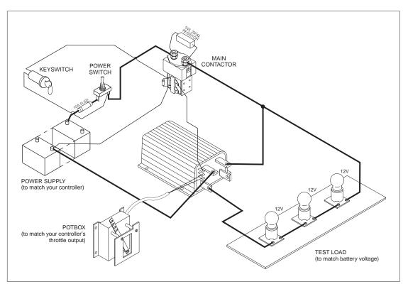
Fig. 19 Setup for bench testing.
