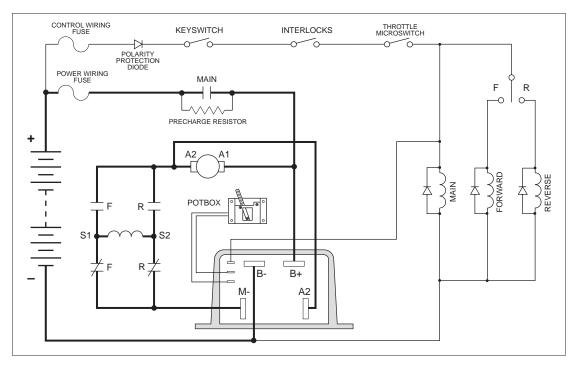
Fig. 9 Basic wiring configuration, Curtis PMC 1209B/1221B/1221C controllers.
