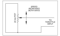
together. The resistance goes from 5  $k\Omega$  at neutral to zero at the extremes: the opposite of the standard throttle input configuration. Contact the factory if you need this type of controller.
