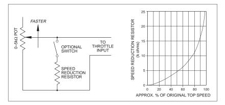
The speed reduction shown in the curve is approximate. The actual vehicle top speed will depend on the motor characteristics and the vehicle load. You should determine by experiment the proper resistor value to give the desired speed reduction. (NOTE: With reduced speed operation, only top speed is reduced; full power is maintained for starting at low speeds.)
