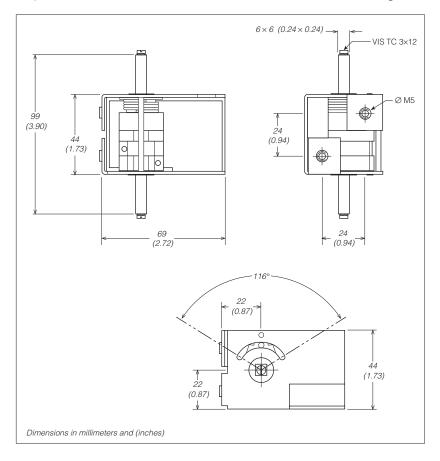
The CH-XXX is a complete control head assembly, consisting of an ET-XXX throttle integrated into a molded steel and plastic assembly designed for mounting directly to the tiller stem of material handling lifts. For more information about ET and CH products, call your local dealer or Curtis office.
