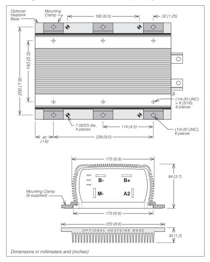
Six mounting clamps are provided, which can be used to attach the controller to its matching heatsink (Curtis PMC p/n 16421001) or to some other surface. An alternative mounting method is provided by six tapped holes on the bottom of the controller. The case outline, heatsink outline, and mounting dimensions are shown in Figure 3.
