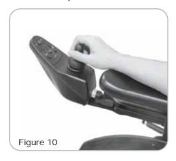
5.Practice driving where there is no obstacle. Start at slowest speed and move forward and backward; make some turns. As you get more comfortable, you can increase the speed by turning speed dial knob clockwise.
