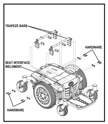
Figure 15. Seat Height/Angle Adjustment
