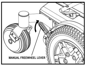
Figure 9. Drive Mode (Drive Engaged)
