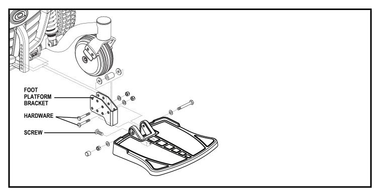
Figure 19. Foot Platform Adjustment
