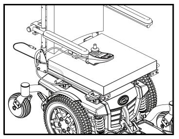
Figure 12. Controller Harness Routing on a Synergy Seat
