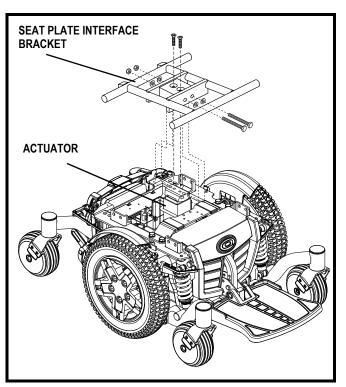
Figure 14. Power Elevating Seat Actuator
