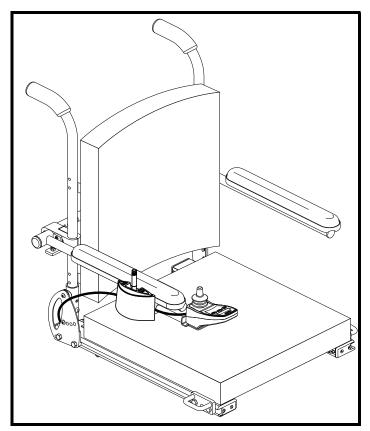
Figure 20. Power Elevating Seat Toggle Switch
