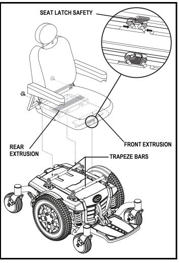
Figure 11. Universal Mounting System and Contour Seat
