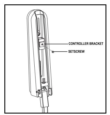
Figure 18. Underside of Armrest
