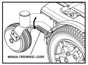
Figure 8. Freewheel Mode (Drive Disengaged)
