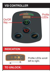
Push joystick forward until beep then pull joystick back until beep. Unit is now unlocked.
